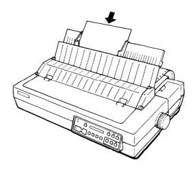
**6.** Press the **LOAD/EJECT** button once to automatically load **the** paper.
